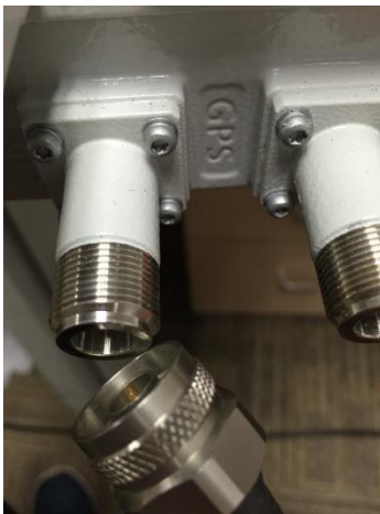
Figure 3-18 GPS Connector Connect to Base Station
