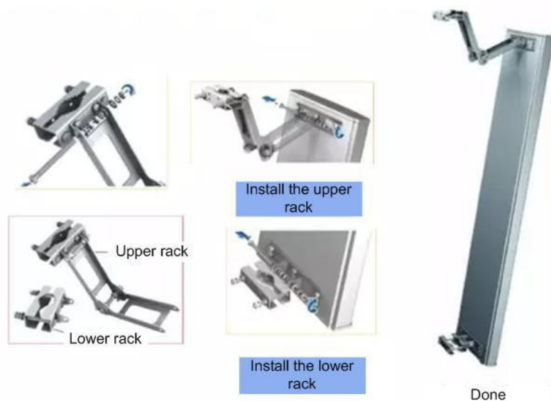
Figure 3-9 Assembling Procedure of Directional Antennas
