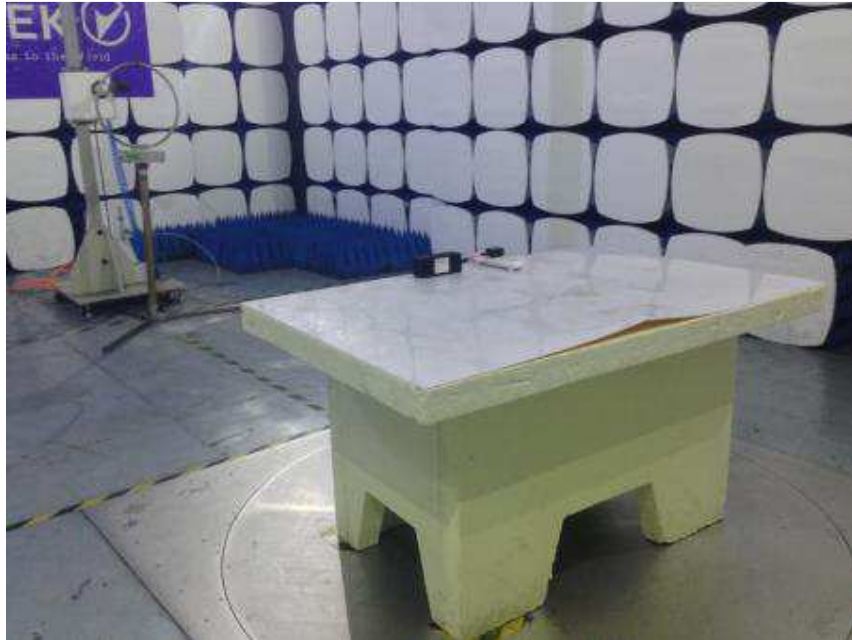
Photograph 2: Set-up for Radiated Spurious Emissions (30MHz-1GHz)
