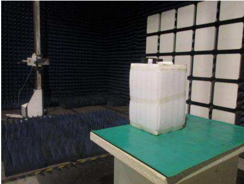
Photograph 4: Set-up for Conducted Emissions
