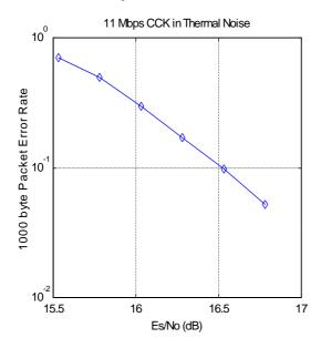
The reference PER is specified as 8%. The corresponding Es/No (signal to noise ratio per symbol) is 16.4 dB. The Es/No required to achieve the desired BER with maximum system implementation losses is 18.4 dB. The minimum processing gain is again, 10 dB, therefore:
