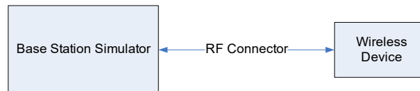
Figure 9-2 Power Measurement Setup
