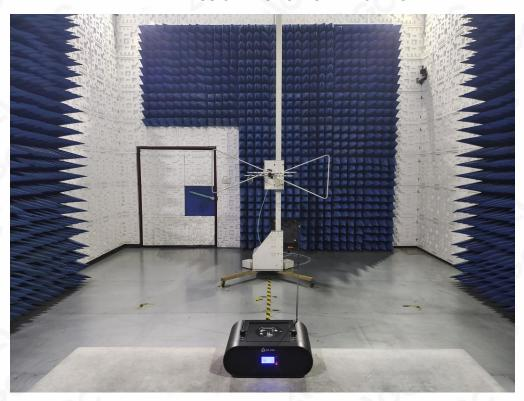
RADIATED EMISSION TEST SETUP ABOVE 1GHz
