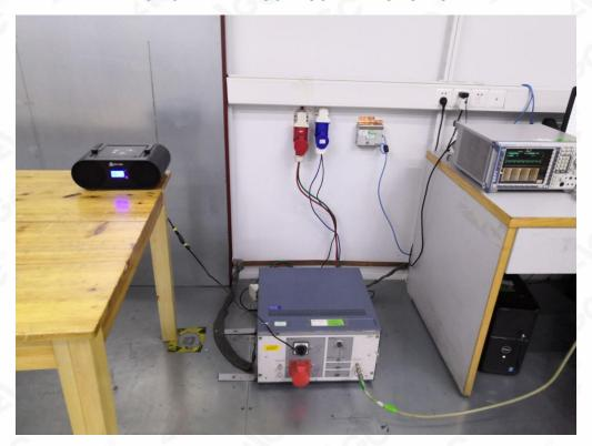
RF CONDUCTED TEST SETUP
