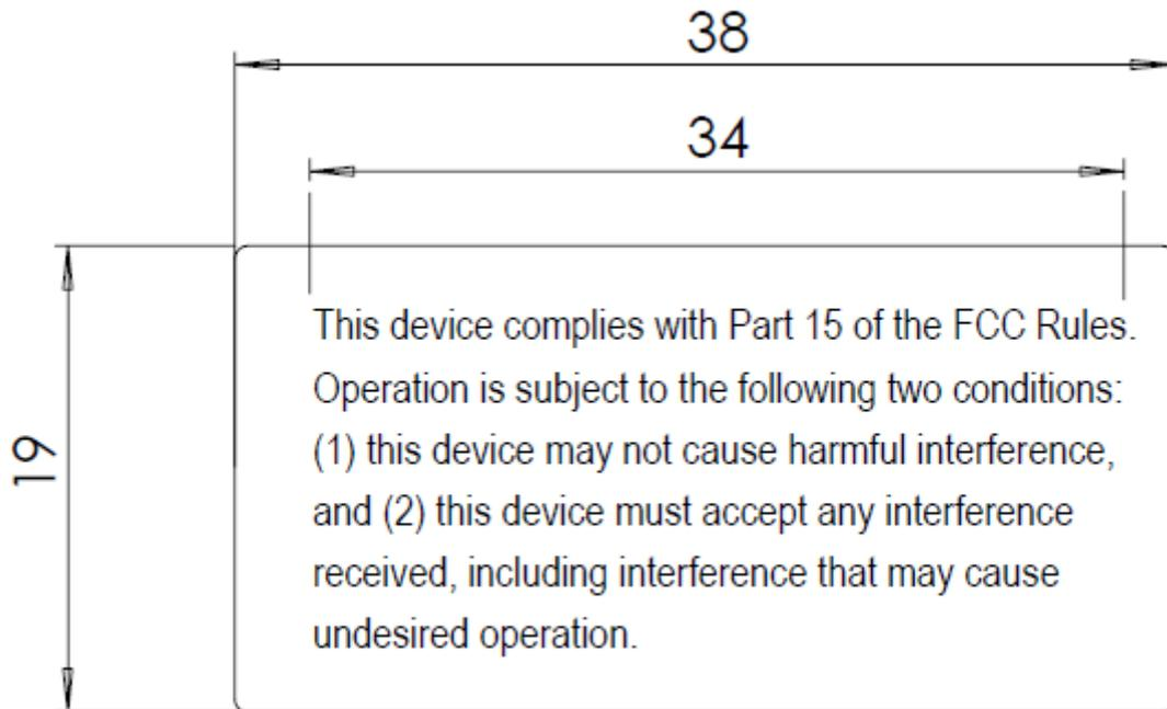
**FCC Part 15B Label - the size of each section is expressed in mm
