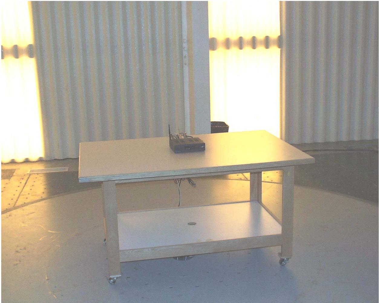
Photograph 1 - Front View Radiated Spurious Emission Worst Case Configuration
