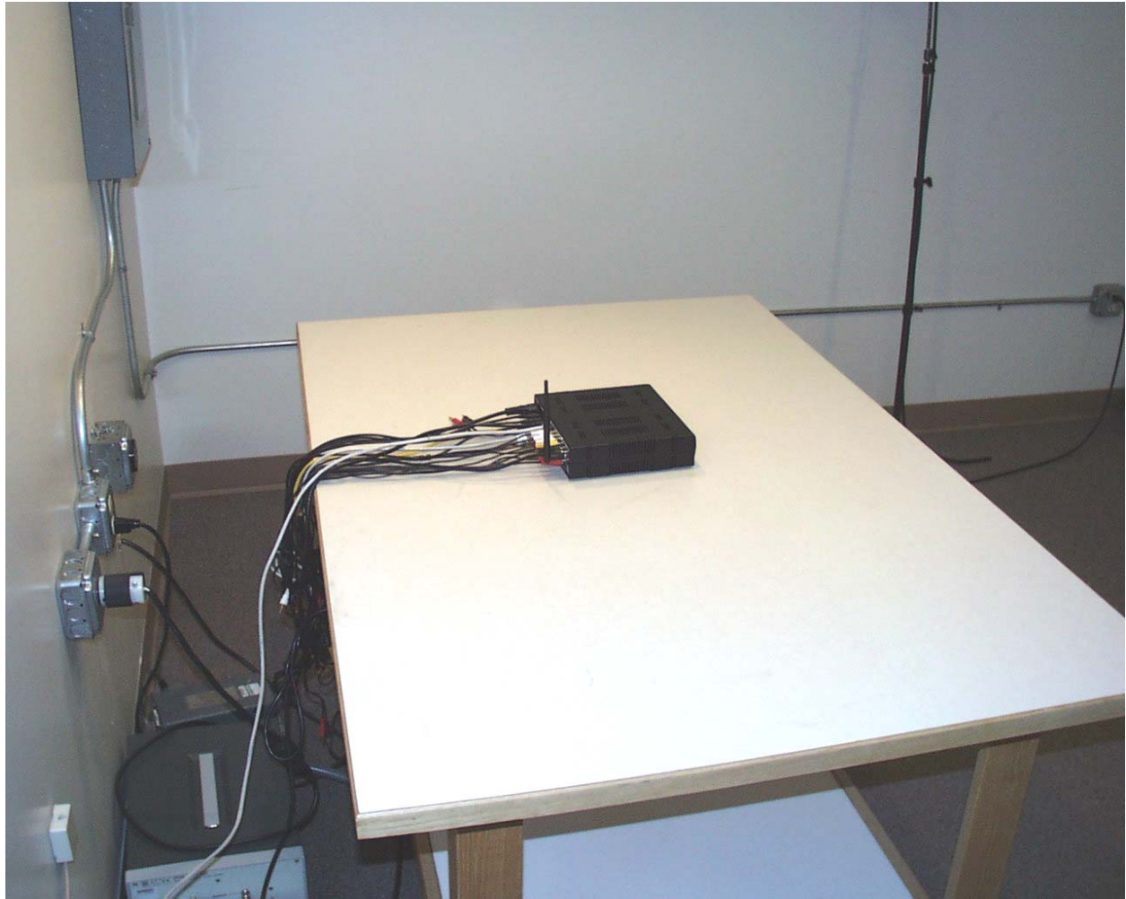
Photograph 4 - Back View Conducted Disturbance Worst Case Configuration
