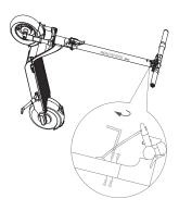
2. Attach the handlebar to the stem
