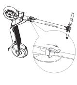
3. Tighten the screws onto both sides of the stem with the hexagon wrench
