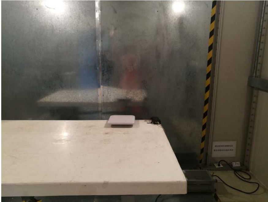
Conducted Emissions (Side View)
