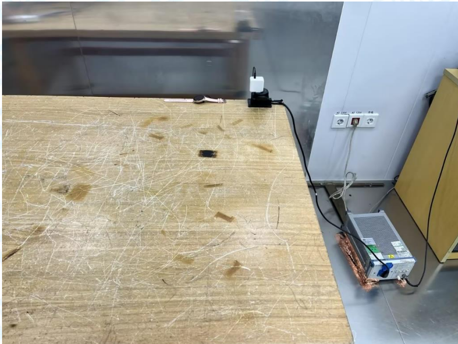
Photo of Setup for Radiated Emission (30MHz~1GHz)
