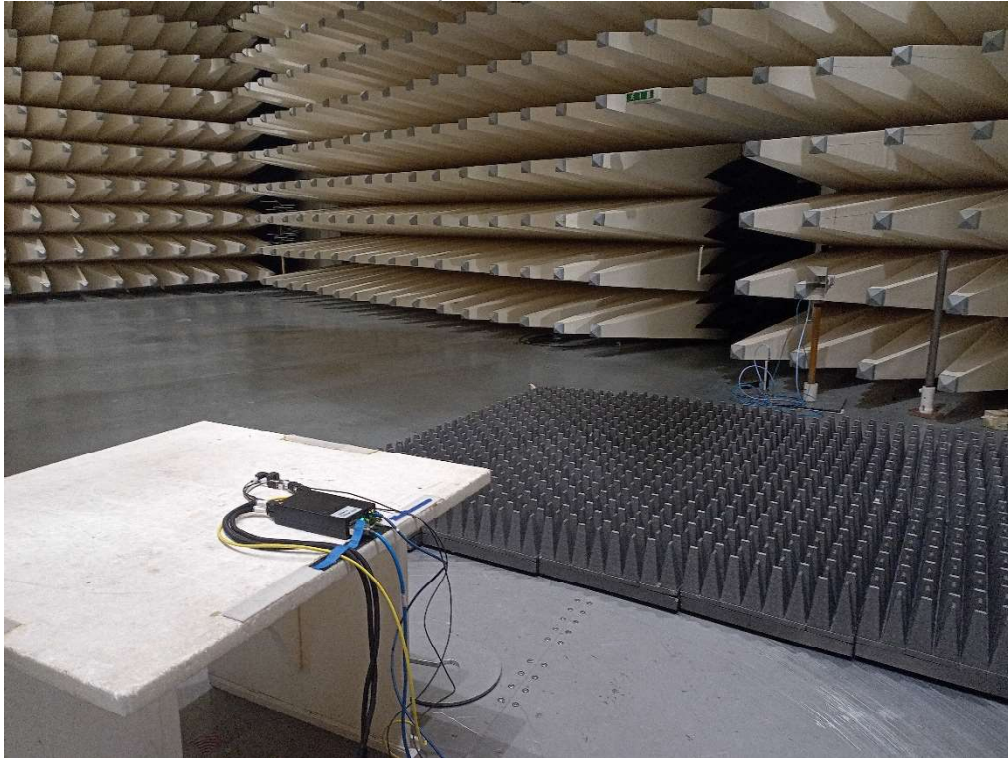
Photo 3: test setup of radiated emission >1GHz
