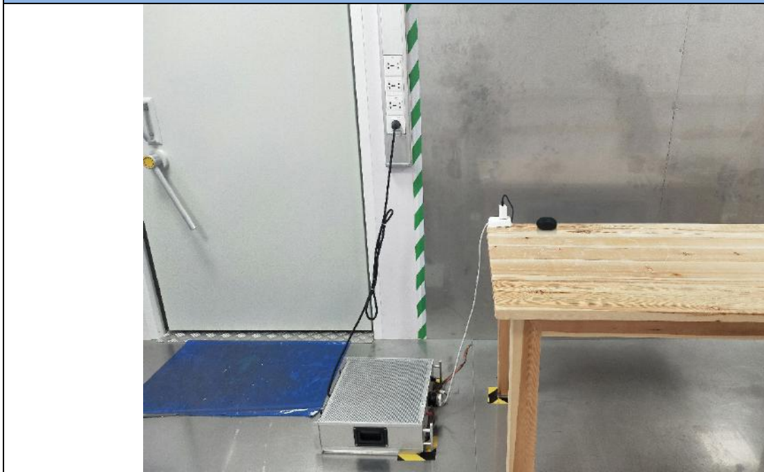
Conducted Emission at AC power line
