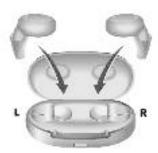
The hearing instruments are automatically turned off and start charging. The charging status is shown for 7 seconds.
