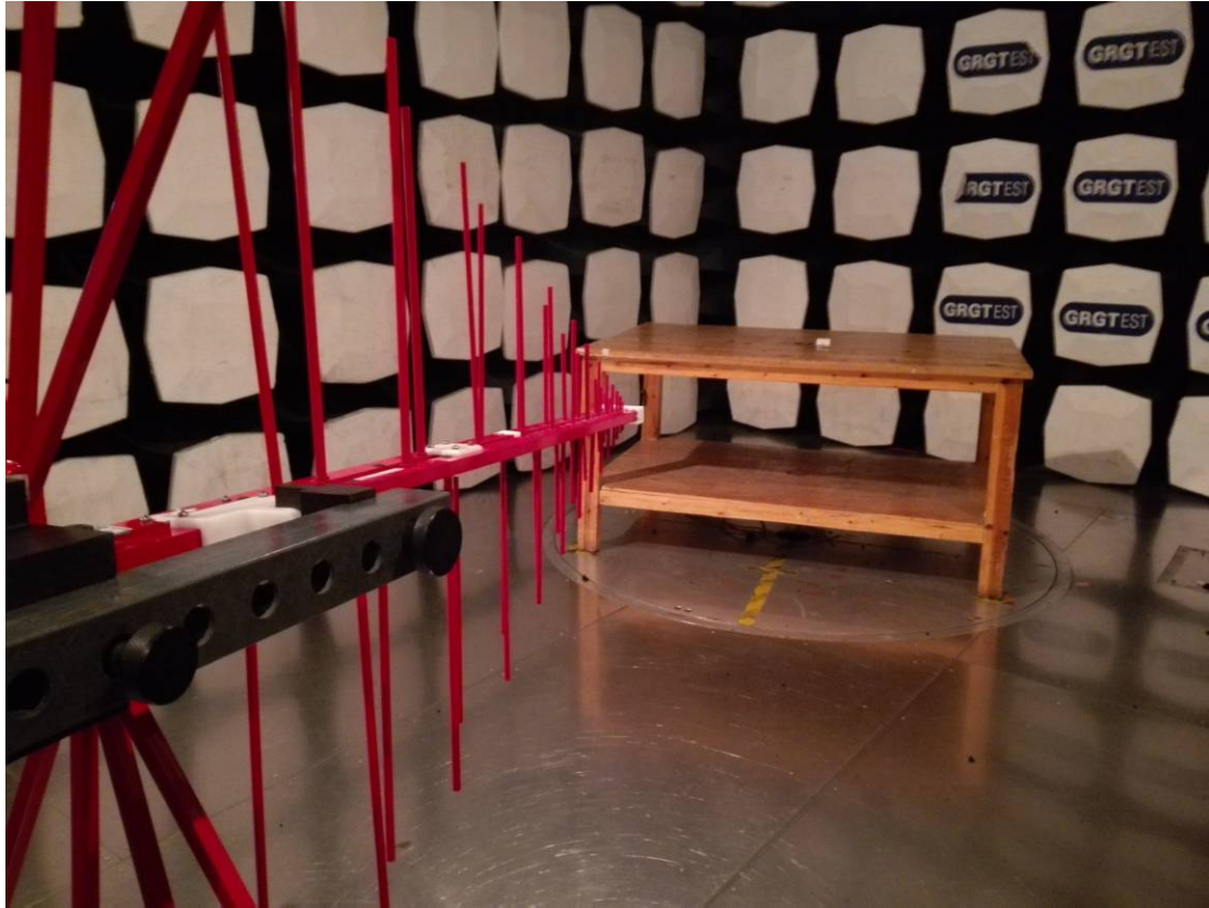
Radiated Emission (Below 1GHZ)
