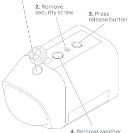
**4.** Remove weather seal, and insert in unused hole
