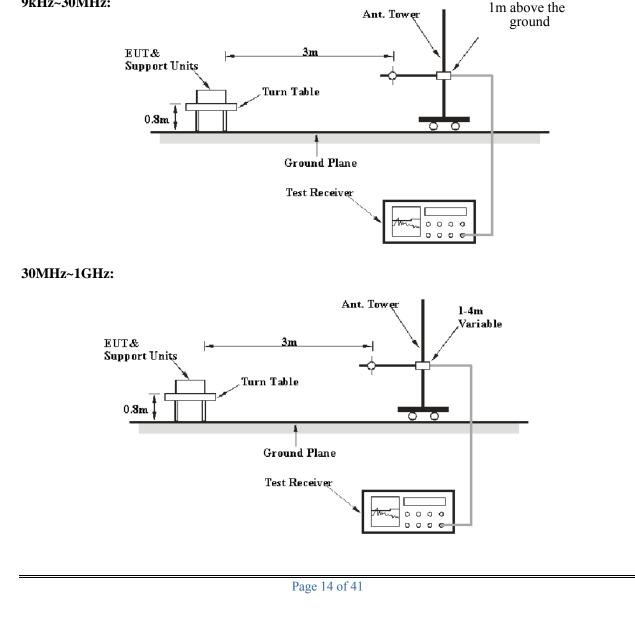
The radiated emission tests were performed in the 3-meter chamber test site, using the setup accordance with the ANSI C63.10-2013.
