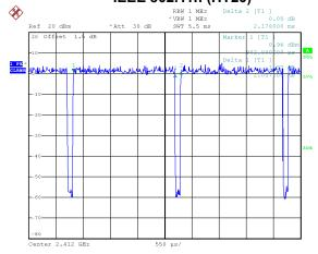
Duty cycle = 2.064 ms / 2.176 ms = 94.85% Duty Factor = 10 log(1/Duty cycle) = 0.23 IEEE 802.11n (HT40)
