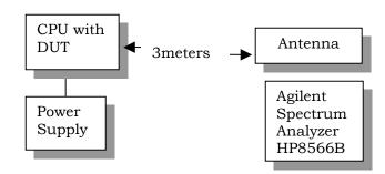
Equipment placed 80cm above ground on a rotating platform.
