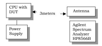
Equipment placed 80cm above ground on a rotatable platform.
