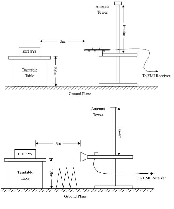
Frequency :9kHz-30MHz RBW=10KHz, VBW =30KHz Sweep time= Auto Trace = max hold Detector function = peak Frequency :30MHz-1GHz RBW=120KHz, VBW=300KHz Sweep time= Auto Trace = max hold Detector function = peak, QP Frequency :Above 1GHz RBW=1MHz, VBW=3MHz(Peak), 10Hz(AV) Sweep time= Auto Trace = max hold Detector function = peak, AV
