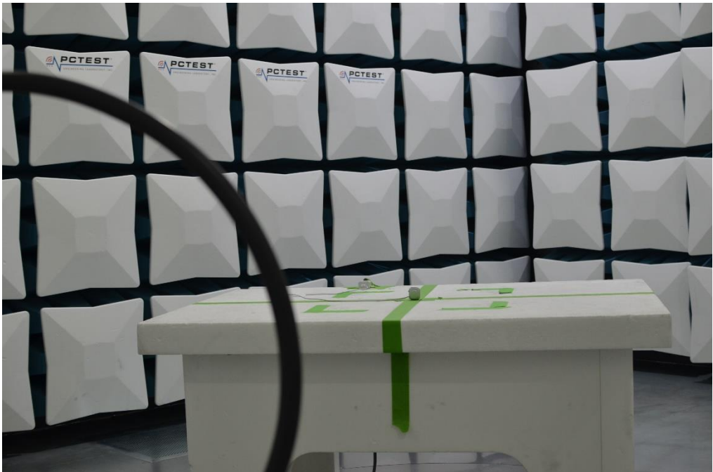
Figure 25: 9kHz-30MHz Test Setup (Front View)
