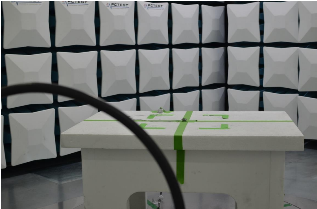
Figure 23: 9kHz-30MHz Test Setup (Front View)
