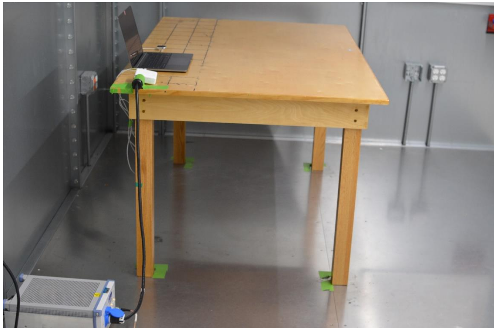
Figure 4: AC Line Conducted Emissions (Side View)
