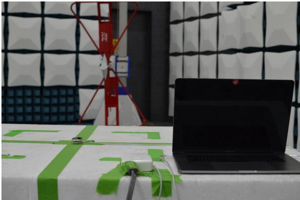
Figure 18: 30MHz-1GHz Test Setup (Rear View)
