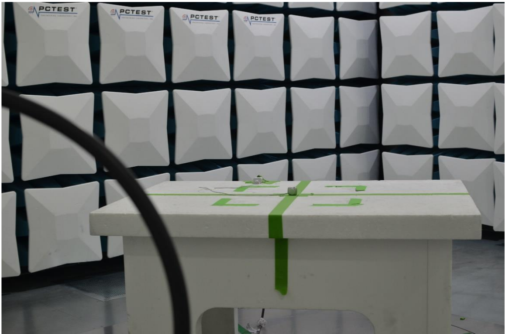
Figure 24: 9kHz-30MHz Test Setup (Front View)
