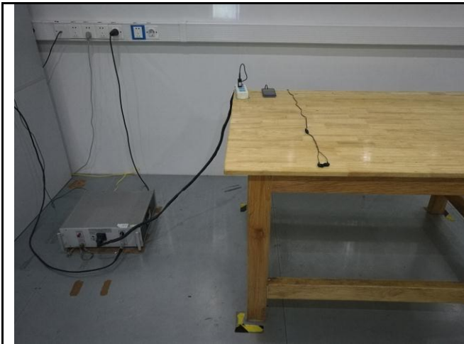
Conducted Emissions Test Setup Front View
