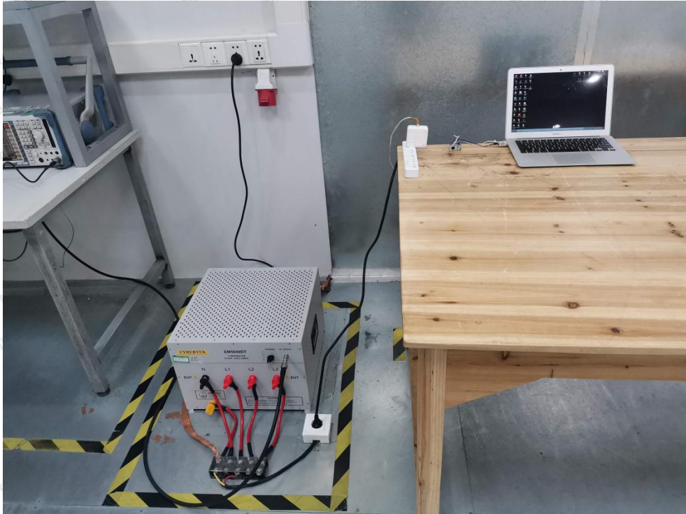
Photo of Power Line Conducted Emission Test
