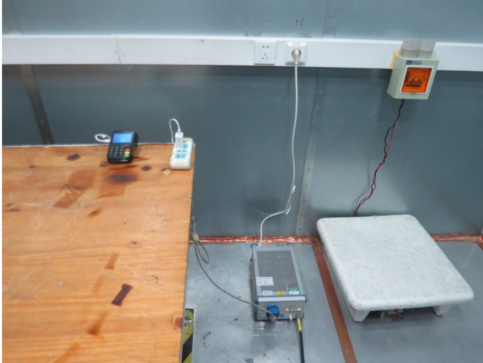
Picture 2 Conducted Emission Test Setup
