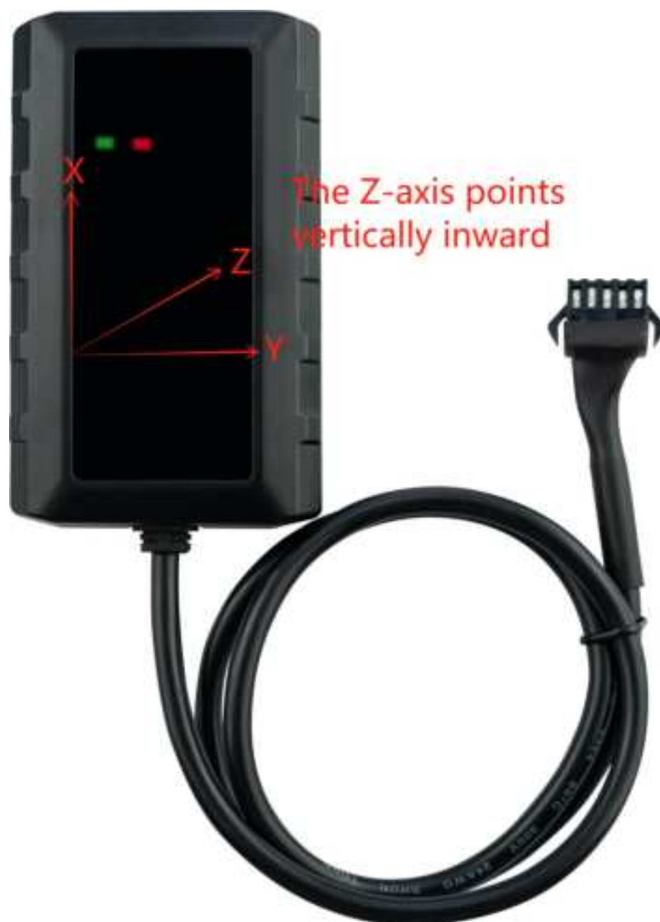
Figure 9. Motion Sensor Direction
