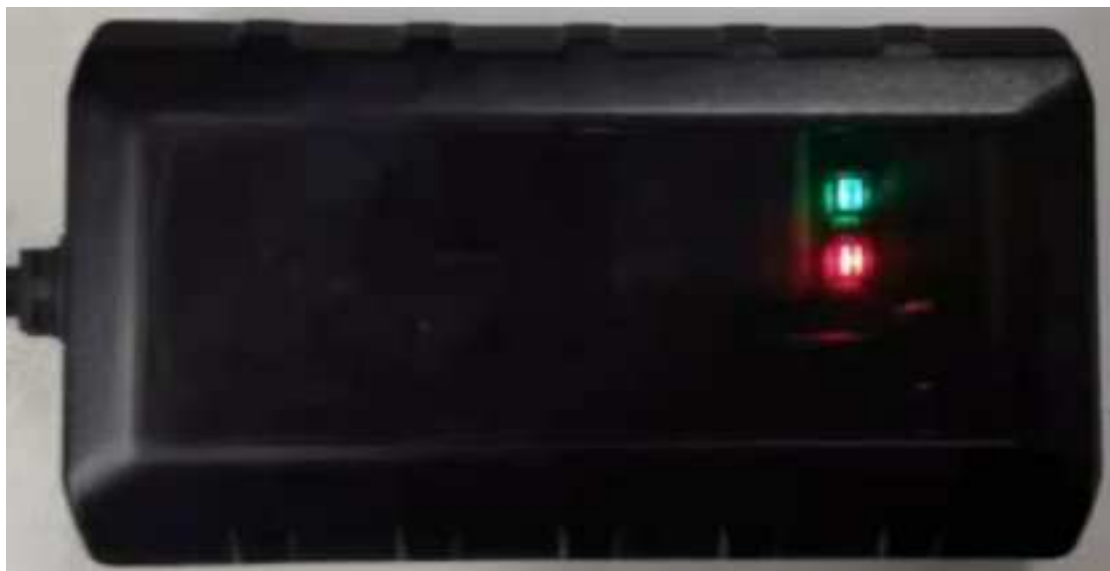
Figure 8. GV57MG V2 LEDs on the Case
