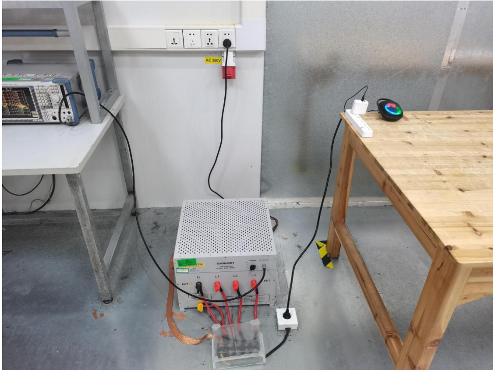
Photo of Conducted Emission Measurement
