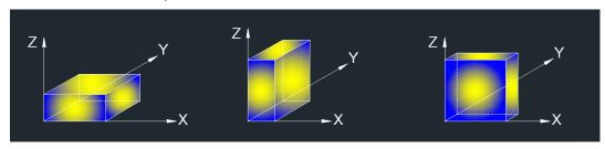
Note: The EUT was investigated in three orthogonal orientations X/Y/Z on ANT0 to determine the worst-case orientation. X orientation is finally determined the worst.
