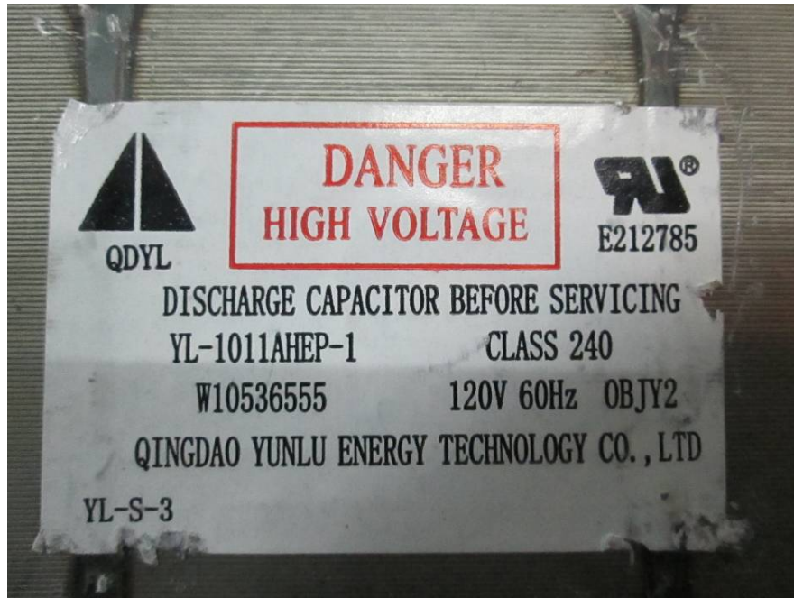
EUT – H.V. Capacitor Label View
