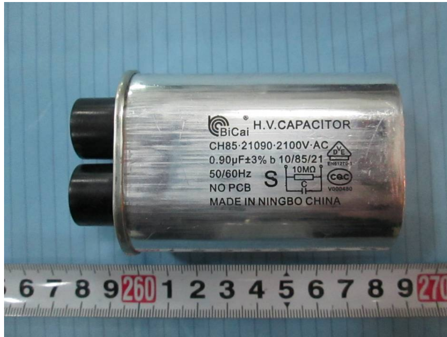
EUT – H.V. Capacitor Front View
