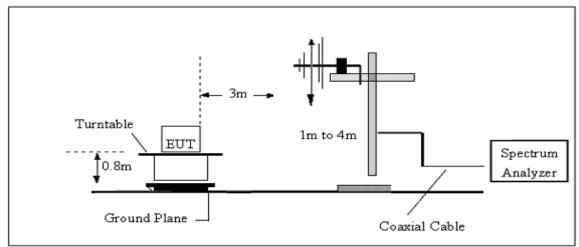
3. Radiated Emission Test-Up Frequency Above 1GHz
