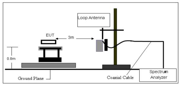
2. Radiated Emission Test-Up Frequency Below1GHz
