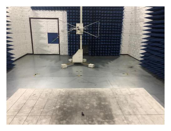
RADIATED EMISSION TEST SETUP ABOVE 1GHZ
