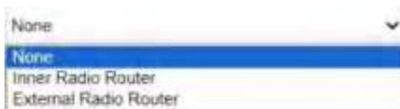
**RadioTransfer:** This is the function that INNO8 is able to transfer the correction from Base station to the other rovers with the internal UHF, definitely, INNO8 can work as a radio transfer (radio repeater).
