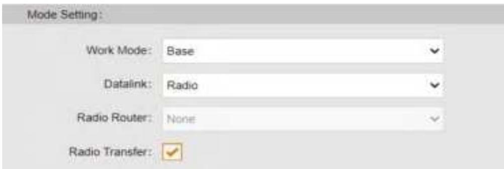
2, open the same function for Rover in critical status (when the Rover is close to working distance of Base internal UHF).
