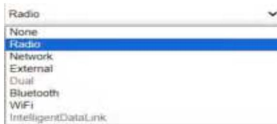
**Radio Route:** This feature is used to transfer the correction which from the reference station to the other rover by radio, the rovers will have the same reference coordinates. This is in the case of working in some places where there is poor signals from reference station or there is only a SIM card for a few rovers. It is able to use internal radio or connect an external radio to transfer the correction. This feature is only available on Rover mode.
