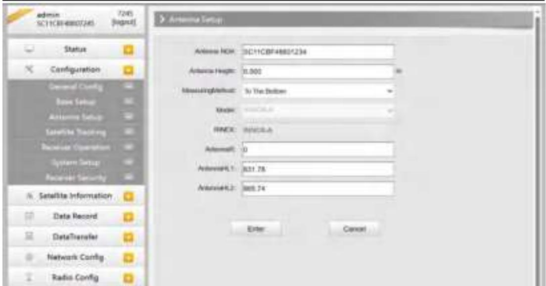
**Antenna Height:** This is the value for height of antenna while surveying.
