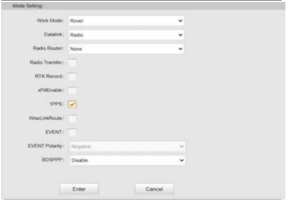
**Work Mode:** There are Rover, Base and Static contained in this dropdown list
