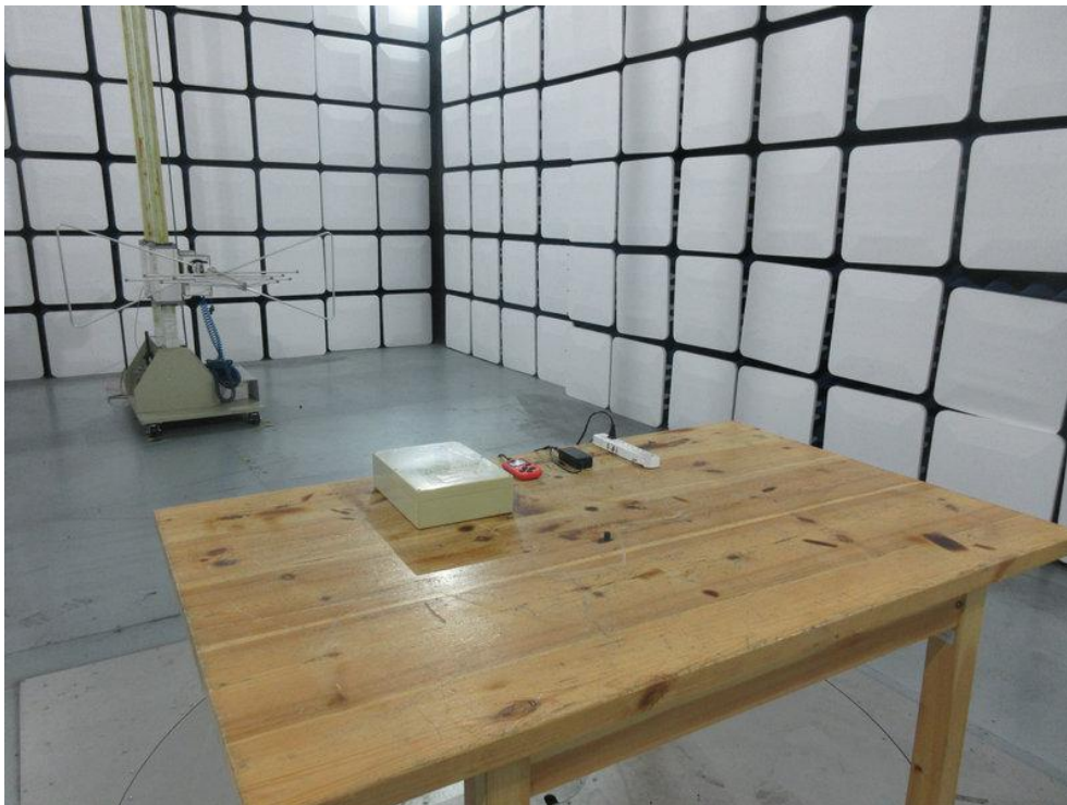
Photo of Radiation Emission Test
