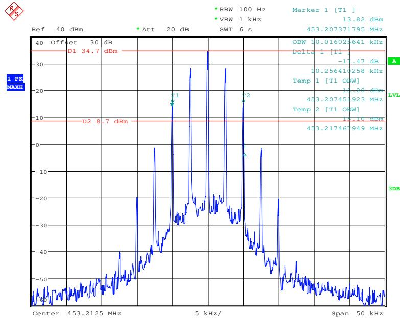
**Frequency 453.2125 MHz: 99% Occupied & 26 dB Bandwidth, Low Power**
