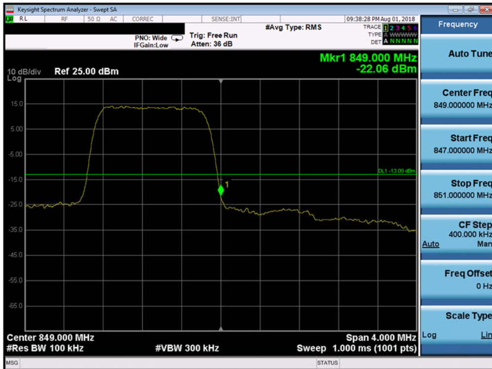
Plot 7-67. Upper Band Edge Plot (Band 26/5 - 1.4MHz QPSK - Full RB Configuration)
