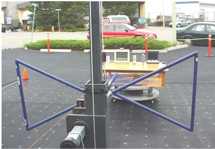
Photograph F-3 - Front of Radiated Emission Configuration
