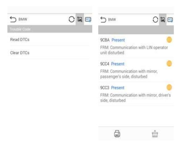
**Freeze Frame** - icon displays when freeze frame data is available for viewing; Tap icon to display data screen. The Freeze Frame interface is similar to that of the Read DTCs interface and share similar operations.
