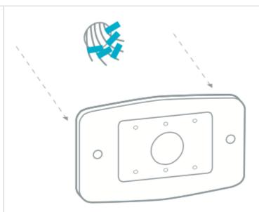
mportant It's important that the power to your system is off to avoid blowing a fuse in your equipment If you blow a fuse, your Nest thermostat won't turn on, or may display a power error after installation.
