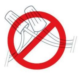
f your thermostat is labeled 120V or 240V or has thick wires with wire nuts, your system is high voltage and isn't compatible with the Nest thermostat. Do not connect the Nest thermostat to high-voltage wires.
