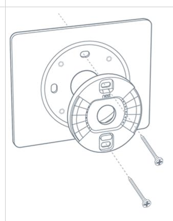
f you're going to use the optional trim plate, place it on the wall before installing the Nest base.
