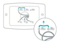
Jumper wires are short wires between two connectors. The Nest thermostat doesn't need them.
