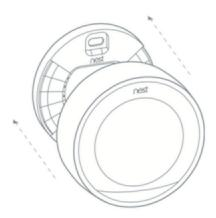
Line up the pin connector on the back of the display and push it onto the base until it clicks into place.
