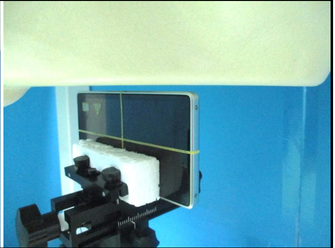
Bottom Side of EUT with 0.5 cm Gap
