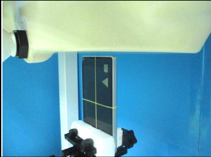
Right Side of EUT with 0.5 cm Gap
