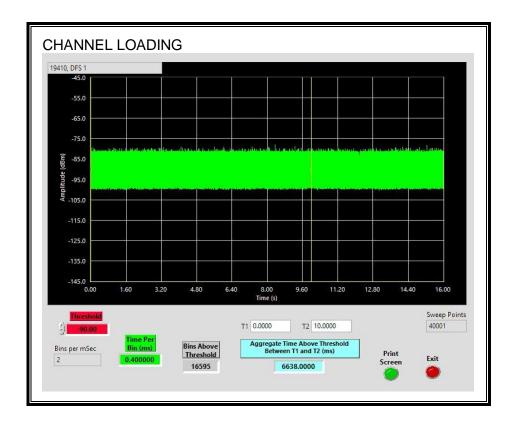
The level of traffic loading on the channel by the EUT is 66.38%
