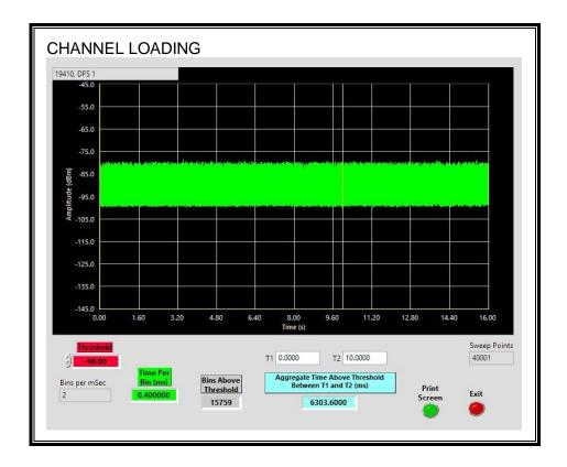
The level of traffic loading on the channel by the EUT is 63.03%
