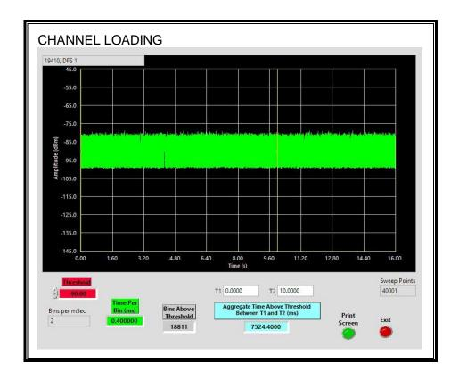
The level of traffic loading on the channel by the EUT is 75.24%
