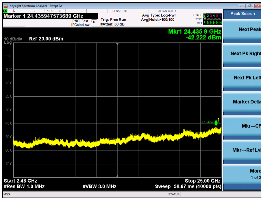
TEST PLOT OF OUT OF BAND EMISSIONS THE WORST CASE OF 802.11n40 FOR MODULATION IN HIGH CHANNEL
