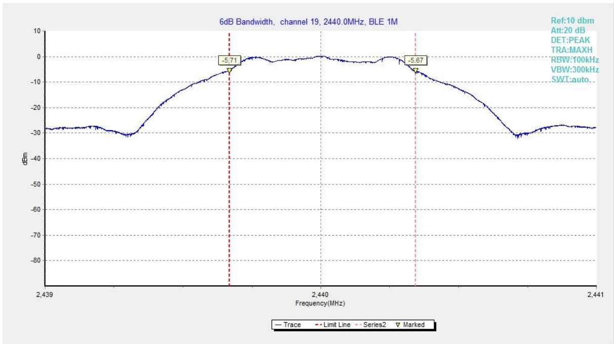
Fig.8 6dB Bandwidth (Ch 19), LE 1M
