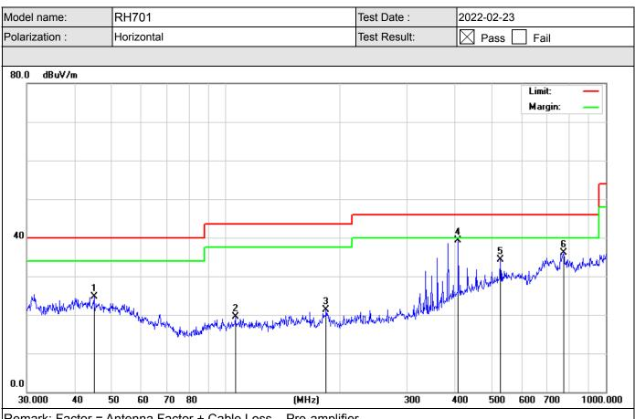
Remark: Factor = Antenna Factor + Cable Loss – Pre-amplifier. Measurement Result=Reading Level +Correct Factor;
