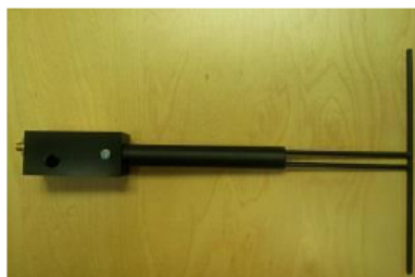
Figure 1 – MVG COMOSAR Validation Dipole
