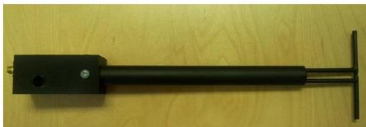
Figure 1 – MVG COMOSAR Validation Dipole
