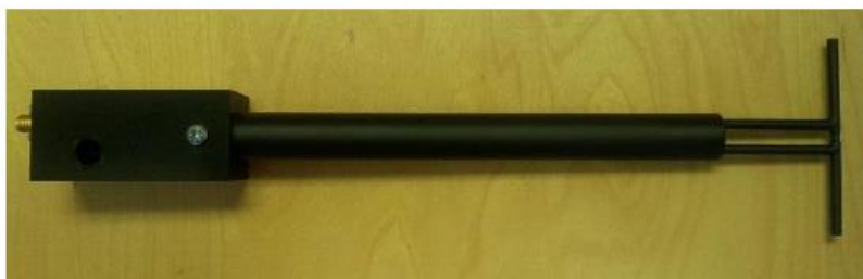
Figure 1 – MVG COMOSAR Validation Dipole
