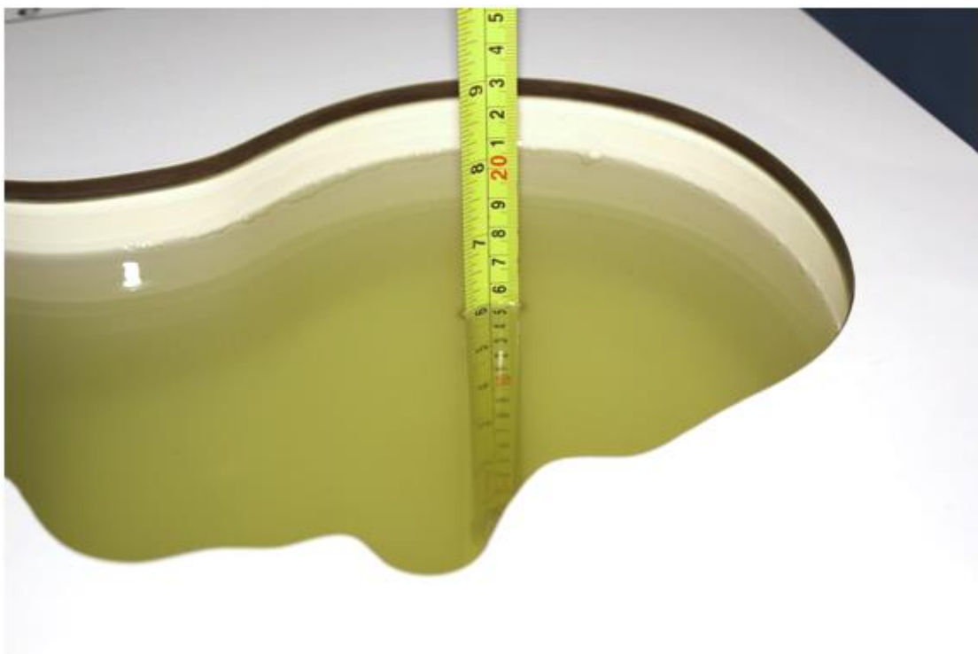
Picture 7-4 Liquid depth in the Head Phantom (2600 MHz)
