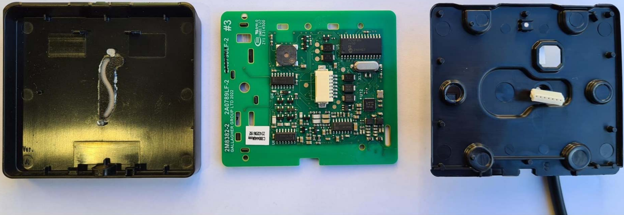
T12 Mifare & Multi Tech - Front/ Back Covers & PCB Assembly
