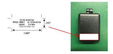
LABEL,FCC, MINI-T LINEAR P/N: 210593 D Mfg, Process: Printed Label or Pad Printing Label Ink: Permanent Black Label Material: Clear Acetate, Adhesive Backed
