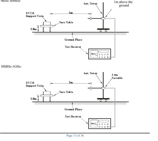
The radiated emission tests were performed in the 3-meter chamber test site, using the setup accordance with the ANSI C63.10-2013.
