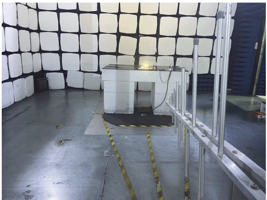
Radiation Emission Test Setup (30MHz to 1GHz)
