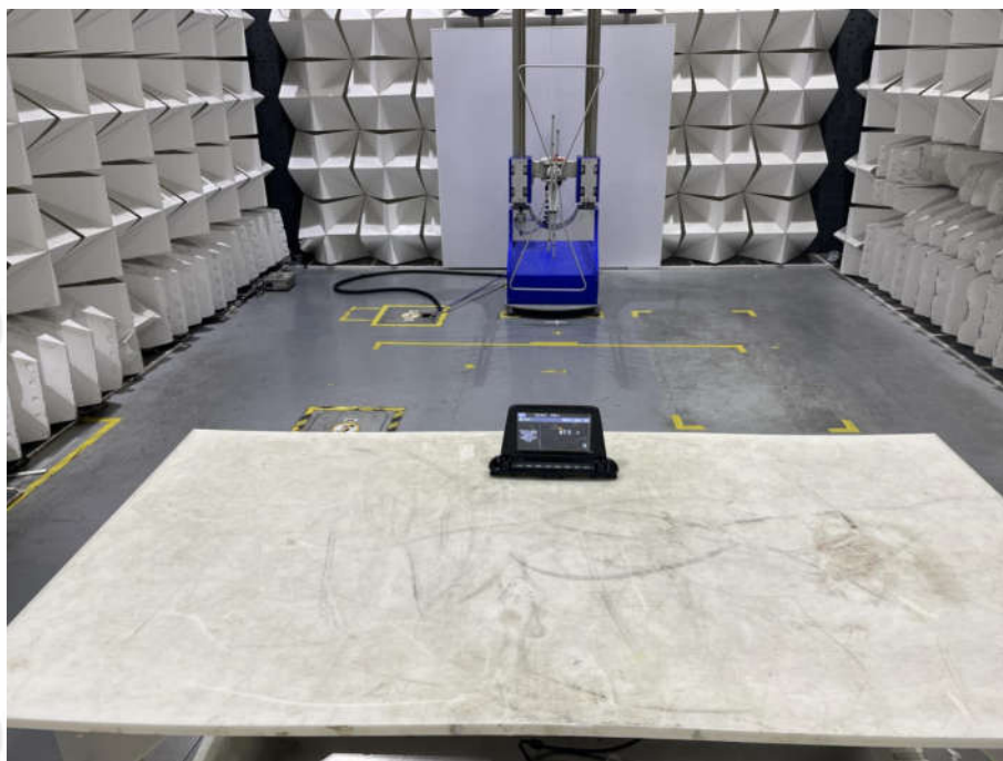
Radiated spurious emission Test Setup-1(Below 1GHz)
