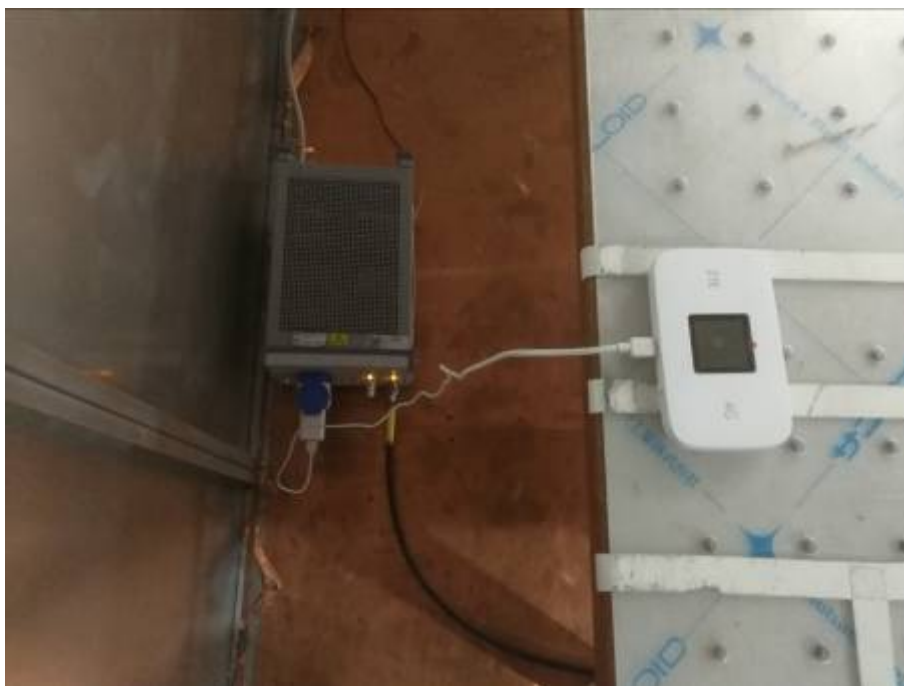
Conducted Emissions Test Setup (with charger)
