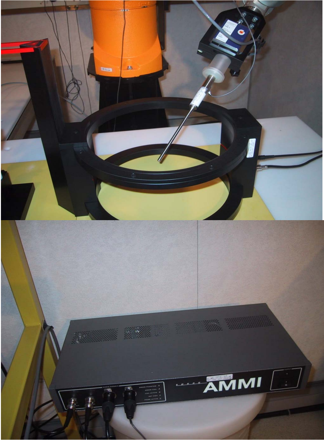
Figure E1: Probe calibration and reference signal measurement setup
